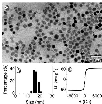
Figure 1. (a) TEM image of the PEG-coated Fe<sub>3</sub>O<sub>4</sub> nanoparticles, (b) size distribution of the particles shown in frame a, (c) room-temperature magnetization curve of the PEG-coated Fe<sub>3</sub>O<sub>4</sub> nanoparticles.
