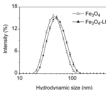
Figure 2. Hydrodynamic size distribution profiles of the PEG-coated Fe<sub>3</sub>O<sub>4</sub> and the Fe<sub>3</sub>O<sub>4</sub>-Lf conjugate.
